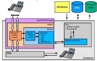
Fig. 5. Combination of firewall and intrusion detection system (bro)
